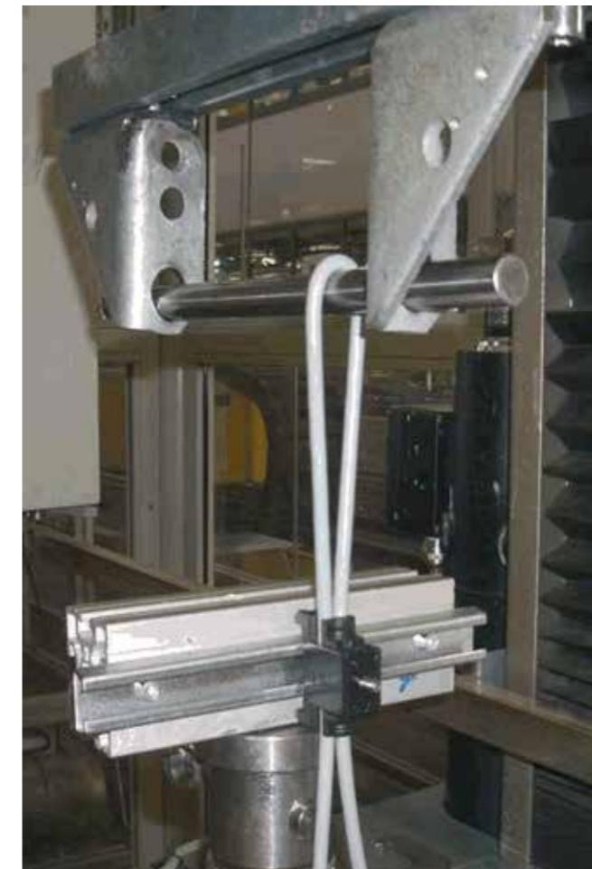
igus® tensile strength test with CFX clamps
