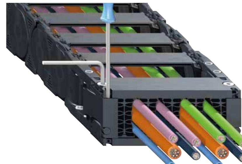
Strain relief can be screwed in from above or below. Compact design is smaller than the mounting bracket of the e-chain® at the fixed end, meaning it can also be used for long travels
